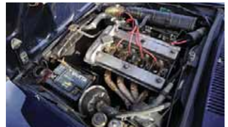
Engine pulls well, showing 80psi oil pressure at 3000rpm
