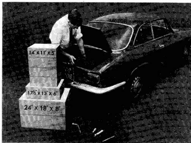
Despite the high sill and slightly narrow boot opening we managed to get a good 6.8 cu.ft. of our test luggage inside. The spare wheel lives under all the luggage. Toolkit is surprisingly versatile.
