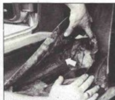
It may only look like superficial rust bubbling (left), but it could mean that the inner section is badly corroded (above left). This is due to a lack of internal body protection and blocked drainage pipes. Peeling back the mats at the door base can reveal a rotten inner sill wall (above right). Also check for rusted seat runners, which can indicate a rotting floor (right). All of this corrosion means a lot of welding and cutting work, which is expensive and time-consuming.
