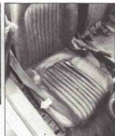
It may only look like superficial rust bubbling (left), but it could mean that the inner section is badly corroded (above left). This is due to a lack of internal body protection and blocked drainage pipes. Peeling back the mats at the door base can reveal a rotten inner sill wall (above right). Also check for rusted seat runners, which can indicate a rotting floor (right). All of this corrosion means a lot of welding and cutting work, which is expensive and time-consuming.
