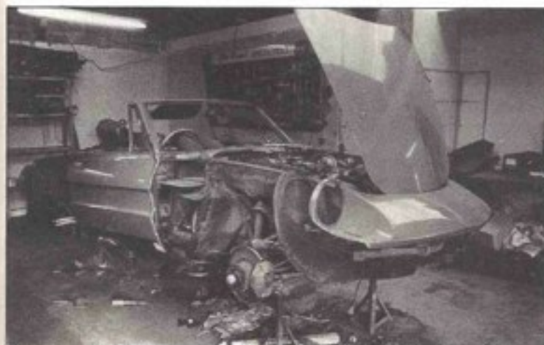
The nightmare of any Spider owner: this low-mileage car needed complete wing replacement
