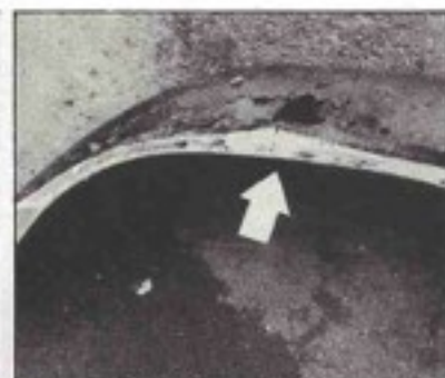
It may only look like superficial rust bubbling (left), but it could mean that the inner section is badly corroded (above left). This is due to a lack of internal body protection and blocked drainage pipes. Peeling back the mats at the door base can reveal a rotten inner sill wall (above right). Also check for rusted seat runners, which can indicate a rotting floor (right). All of this corrosion means a lot of welding and cutting work, which is expensive and time-consuming.
