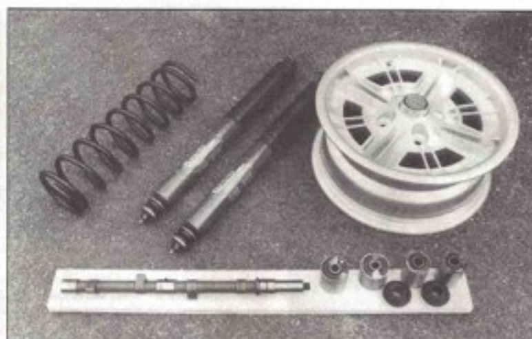
A variety of performance extras: Melba alloy rims, high-lift camshaft, stiffer dampers etc
