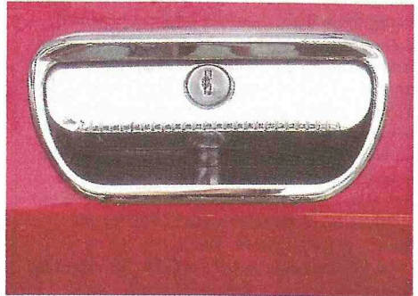
Door handles are sometimes found awkward to use and break. Can weaken steel around them, causing rust
