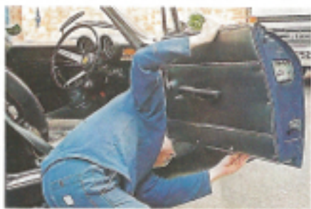
Check all three drain holes are present and there's a neat folded edge all round.
