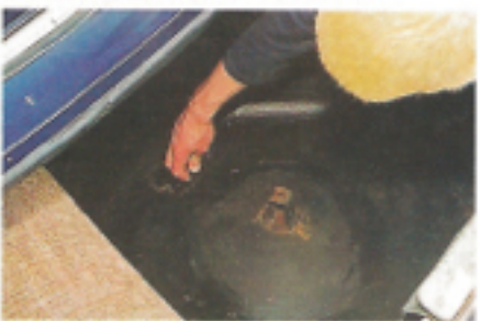
In the boot, pull out the spare wheel and check well, especially around drain holes.
