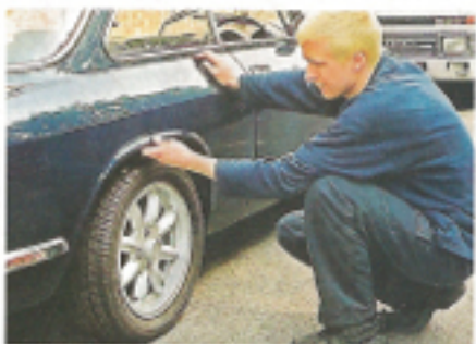
Round profile to arch lip means a replacement. Feel behind it for quality of repair.
