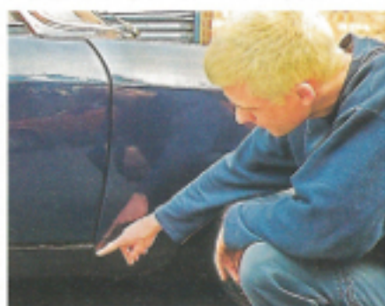
No clear seam where wings overlap the sill means car has been bodged in some way.
