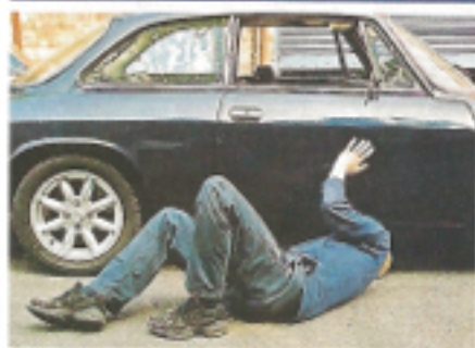
You've really got to inspect the inner sill area. Get under the car and look outwards.
