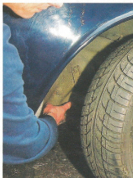
Steering box mounting area cracks. View damage or repairs from driver's side arch.
