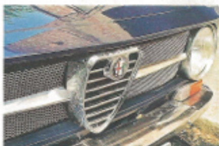
Heart-shaped grilles suffer from pitting, new replacements cost close on £100.
