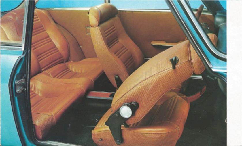
modate two passengers in comfort. The driving position is of the latest design, adopting the central console style which houses the gear lever, water temperature and fuel gauges and the fresh air heating, and ventilation controls as well as switches for the 2 speed windscreen wipers, dash-board light and 2 speed booster fan.
