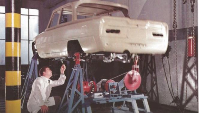
The bodywork, too, is tested. And that of the Giulia is capable of withstanding the severest « torsion stresses ».
