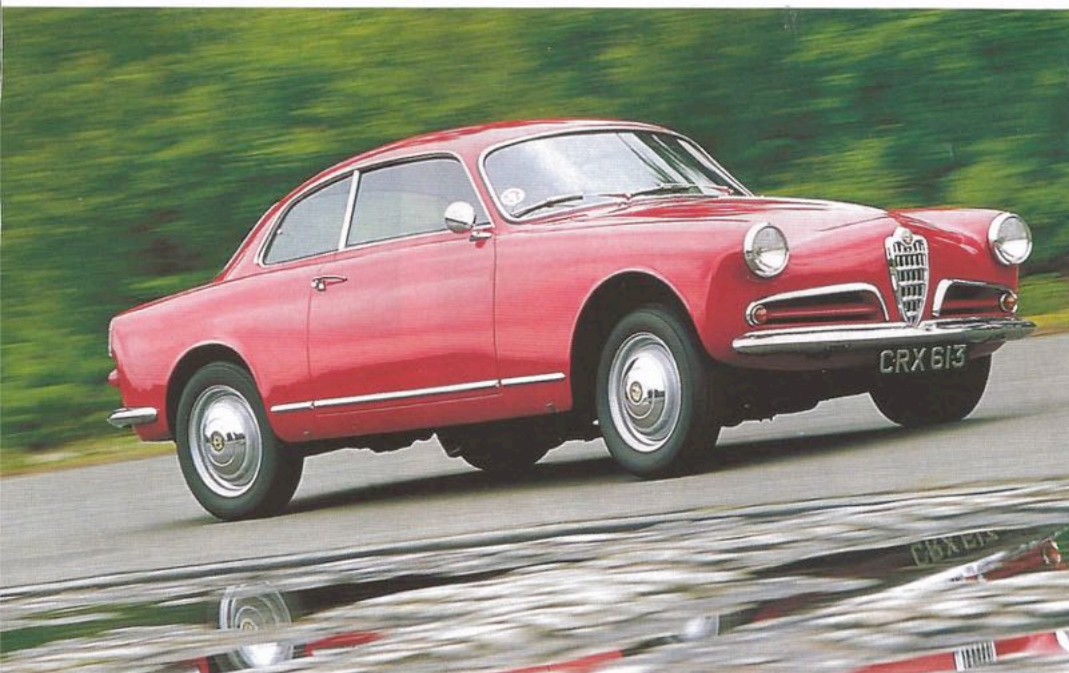
Above: early 750-series Sprint is the oldest in UK; 1290cc alloy twin-cam derived from 1900 unit. Left: each of this diverse family has ardent fans
