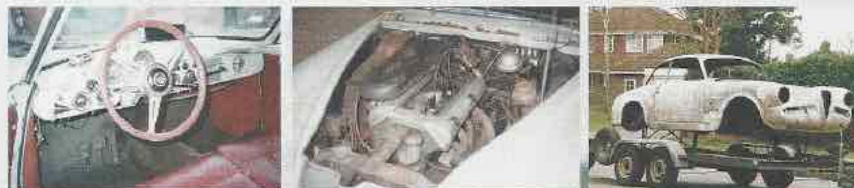
Left to right: the dashboard was covered in non-original gauges and switches before restoration; the seized engine had the wrong camshafts; the stripped body is transported to the paint shop
