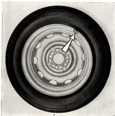
Tabs and plates for static wheel-balancing
