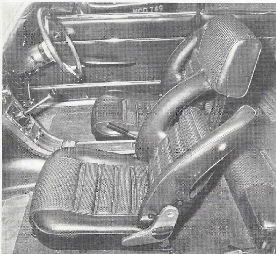
The front seats—grooved and cut away for ventilation—can be reclined and have a good range of fore and aft adjustment. The front passenger's seat has a built-in headrest.
